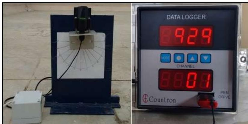
Figure-2: Pyranometer with data logger
